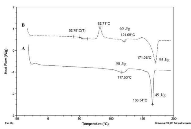
*Figure 2.* DSC thermograms of poly[ethylene-*block*-(L,L-lactide)] block copolymers obtained after a polymerization time of 1 h (A) and 5.67 h (B) (see Table 1; heating rate:  $10^{\circ}$ C · min<sup>-1</sup> under N<sub>2</sub> flow,  $2^{nd}$  scan).
