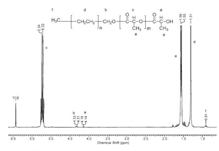
*Figure 1.* <sup>1</sup>H NMR spectrum of poly[ethylene-*block*-( $\iota$ , $\iota$ -lactide)] block copolymer as obtained after 1 h (entry 1, Table 1; solvent =  $C_2D_2CI_4$  at 120 °C).
