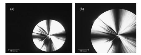
Figure 4. Light microscopy image of a growing PLA spherulite (entry 3) at 140 °C at two different times (20 (a) and 30 sec (b)).
