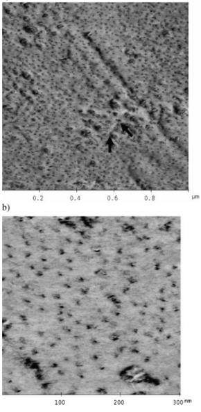
*Figure 3.* AFM phase images of poly[ethylene-*block*-(L,L-lactide)] block copolymer (Table 1, entry 3). Some PE lamellae are marked by arrows.
